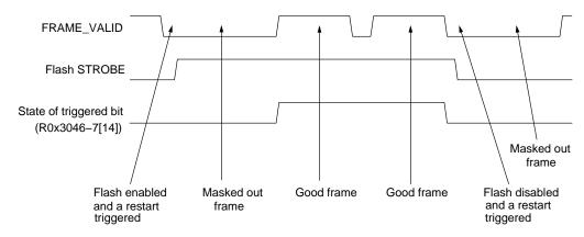
Figure 45. LED Flash Enabled Following Forced Restart
