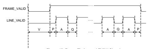
Figure 17. Frame Timing and FV/LV Signals
