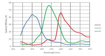
Figure 66. Quantum Efficiency
