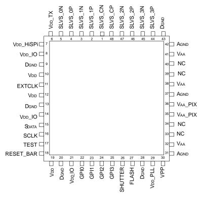
Figure 7. 48-Pin ILCC HiSPi Package Pinout Diagram
