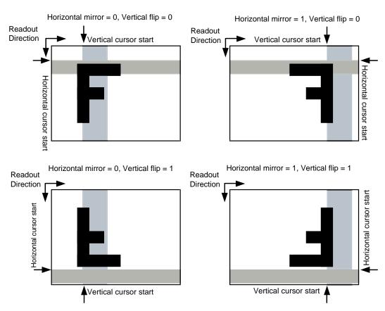
Figure 61. Test Cursor Behavior with Image Orientation
