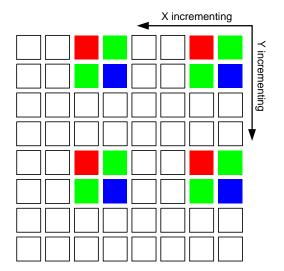
Figure 35. Pixel Readout (x\_odd\_inc = 31, y\_odd\_inc = 3)
