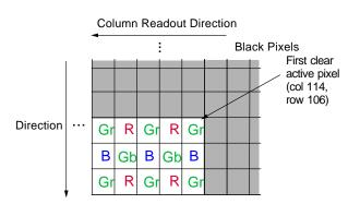
Figure 3. Pixel Color Pattern Detail (Top Right Corner)
