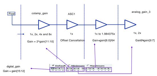
Figure 42. Analog Gain Stages
