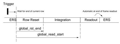
Figure 48. Controlling the Reset and Integration Phases of the Global Reset Sequence
