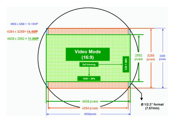
Figure 4. High-Resolution Still Image Capture + HD Video
