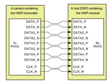
Figure 10. HiSPi Transmitter and Receiver Interface Block Diagram
