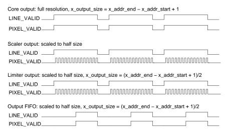
Figure 25. Timing of Data Path
