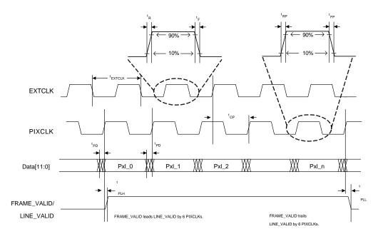
Figure 68. I/O Timing Diagram
