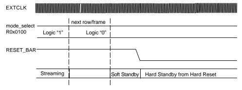
Figure 64. Hard Standby and Hard Reset
