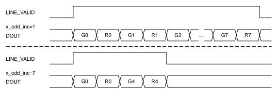
Figure 31. Effect of x\_odd\_inc = 7 on Readout Sequence
