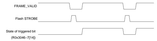
Figure 43. Xenon Flash Enabled
