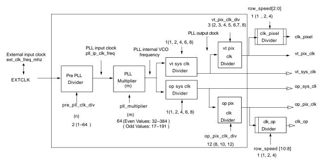
Figure 27. Clocking Configuration
