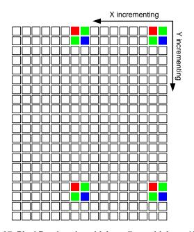
Figure 37. Pixel Readout (x\_odd\_inc = 7, y\_odd\_inc = 15)
