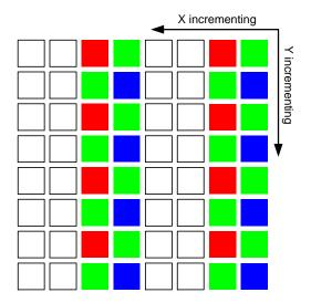
Figure 33. Pixel Readout (x\_odd\_inc = 3, y\_odd\_inc = 1)
