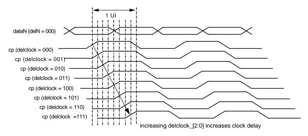
Figure 13. Delaying the clock\_lane with Respect to data\_lane
