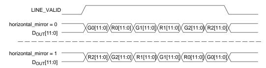
Figure 28. Effect of Horizontal Mirror on Readout Order
