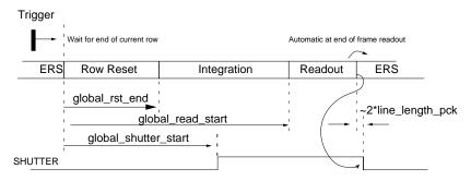
Figure 50. Controlling the SHUTTER Output
