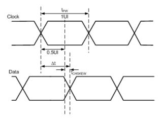
Figure 71. Clock-to-Data Skew Timing Diagram
