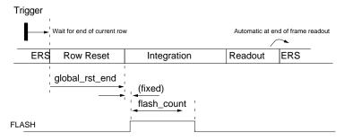
Figure 51. Using FLASH with Global Reset
