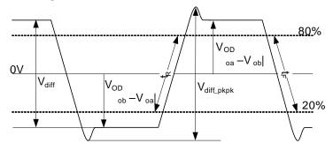
Figure 69. Single-Ended and Differential Signals
