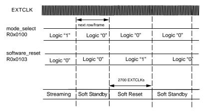
Figure 65. Soft Standby and Soft Reset
