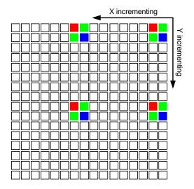
Figure 36. Pixel Readout (x\_odd\_inc = 7, y\_odd\_inc = 7)
