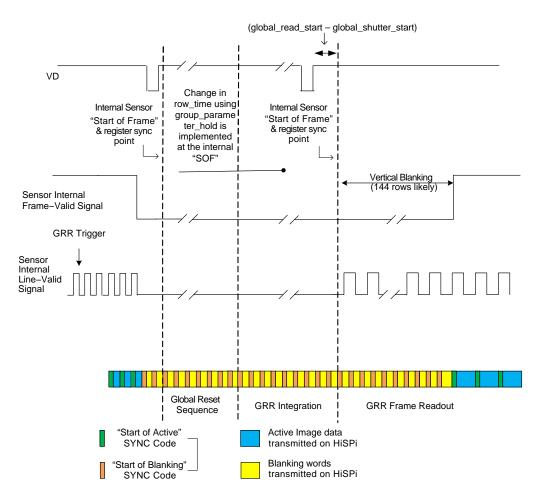
Figure 55. Slave Mode HiSPi Output (ERS to GRR Transition)
