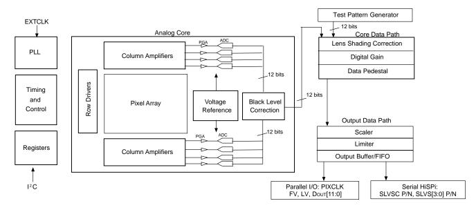
Figure 1. MT9F002 Block Diagram
