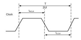
Figure 74. Clock Duty Cycle
