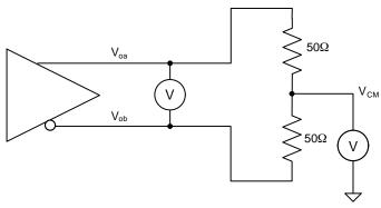
Figure 70. DC Test Circuit
