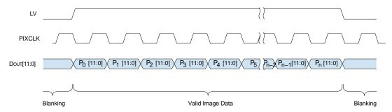
Figure 16. Pixel Data Timing Example
