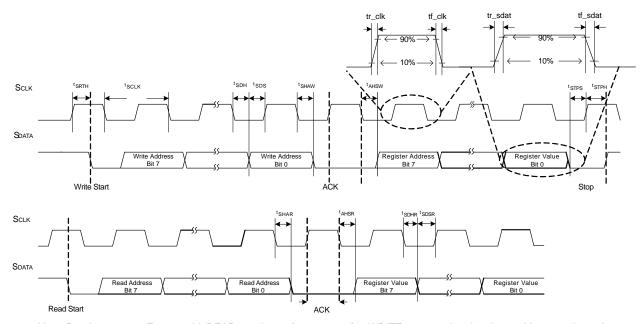
Note: Read sequence: For an 8-bit READ, read waveforms start after WRITE command and register address are issued.
