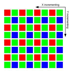
Figure 32. Pixel Readout (No Subsampling)
