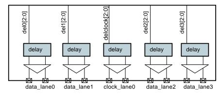
Figure 12. Block Diagram of DLL Timing Adjustment
