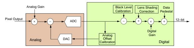
Figure 2. Data Flow Diagram
