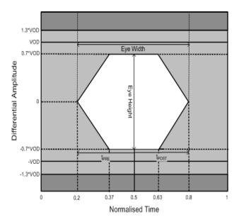
Figure 73. Transmitter Eye Mask
