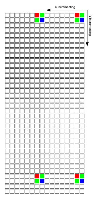
Figure 38. Pixel Readout (x\_odd\_inc = 7, y\_odd\_inc = 31)
