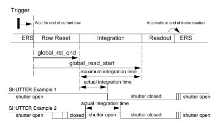
Figure 49. Control of the Electromechanical Shutter
