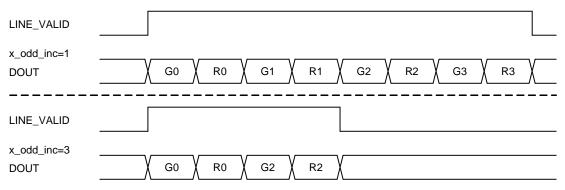
Figure 30. Effect of x\_odd\_inc = 3 on Readout Sequence
