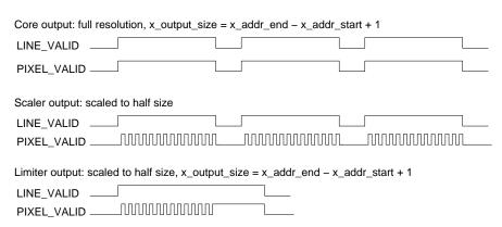
Figure 24. Effect of Limiter on the Data Path
